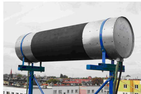
Fig. 1. Scheme of heat exchange on external surface of the pipeline and experimental station in open air space; 1-external shell, 2-sky, 3-bottom, 4-thermal insulation, 5-fluid inside the pipeline
